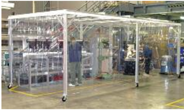
This modular enclosure can be moved throughout a factory to contain specific processes that require a higher degree of protection against contamination. Cleanrooms and enclosures should be in place and the HEPA filters operating for 24 hours to insure proper levels.
